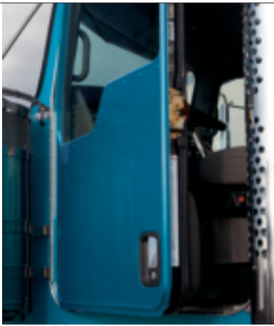
Thick bulkhead-type doors hang on continuous stainless steel piano hinges – not typical automotive hinges – and fit snugly to become an integral part of the cab structure – another reason Kenworth trucks bring more at resale than just about any other make you can name.
