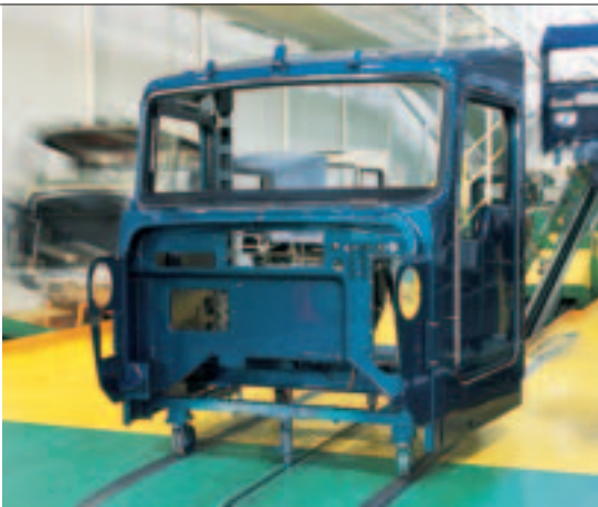
Coil-coated aluminum panels and a one-piece fiberglass roof, supported by an aircraft-grade aluminum alloy frame, produce a lightweight yet durable cab that is virtually immune to corrosion.
