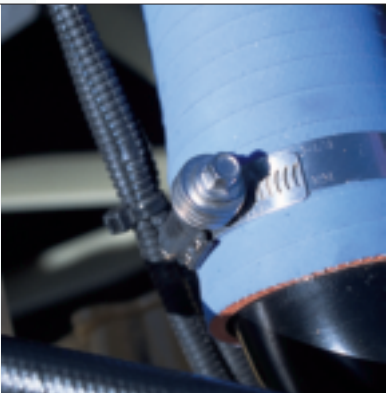
Constant torque hose clamps – standard on Kenworth trucks – go on tight and stay that way.
