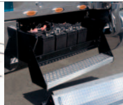
Here is another reason Kenworths are so dependable: 12-volt maintenance-free batteries, held firmly in place and mounted on the left-hand side, close to the starter motor for minimum voltage drop.
