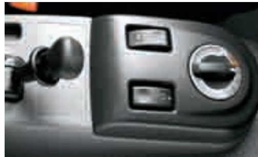
The AS-Tronic control panel is located on the console next to the driver's seat.
